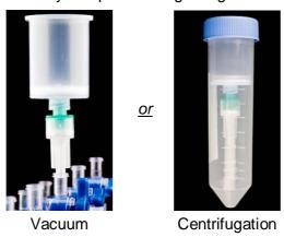
The Zymo-Midi Filter™ attaches to the Zymo-Spin™ V-E spin column for lysate pre-clearing using a vacuum manifold or centrifuge (see pictures above). The Zymo-Midi Filter™ is removed from the spin column for washing and elution steps.
