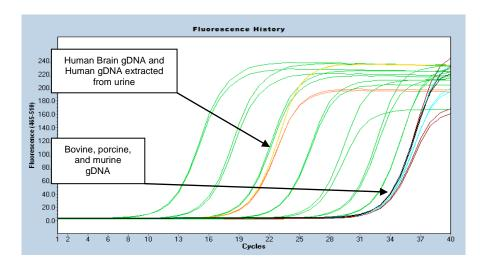
**Specificity:** Amplification plots demonstrate the specificity of the Femto<sup>™</sup> Human DNA Quantification Kit. Bovine gDNA, porcine gDNA, and murine gDNA exhibited delayed amplification similar to the No Template Control (black) (≥35 cycles). 0.2 ng of human brain gDNA (orange), human gDNA extracted from urine (gold), bovine gDNA (red), porcine gDNA (light blue), and murine gDNA (purple) were used.
